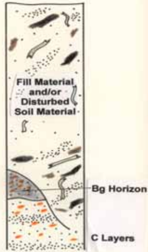
Buried Inplace Soil/Geologic Material with Redox features (inconclusive)
