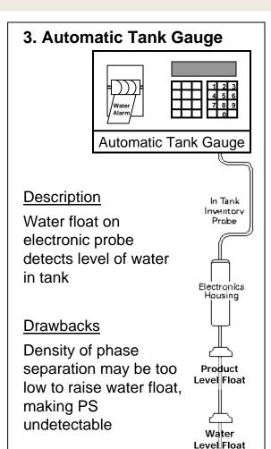
Most water floats were designed for water. However, with the introduction of ethanolblended gasoline, seldom will you have pure water at the bottom of a tank.
