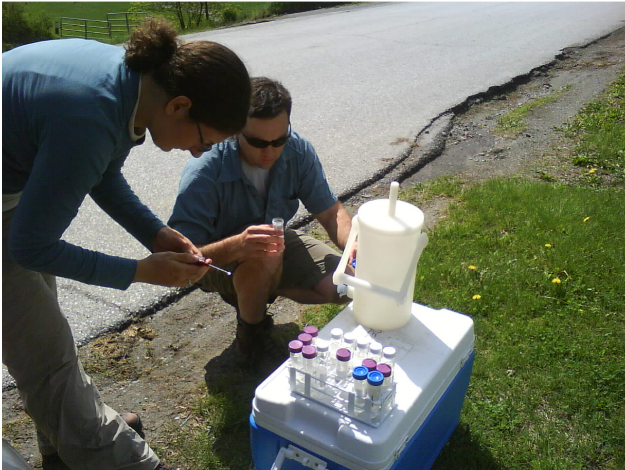
Use of churn splitter to homogenize manual samples
