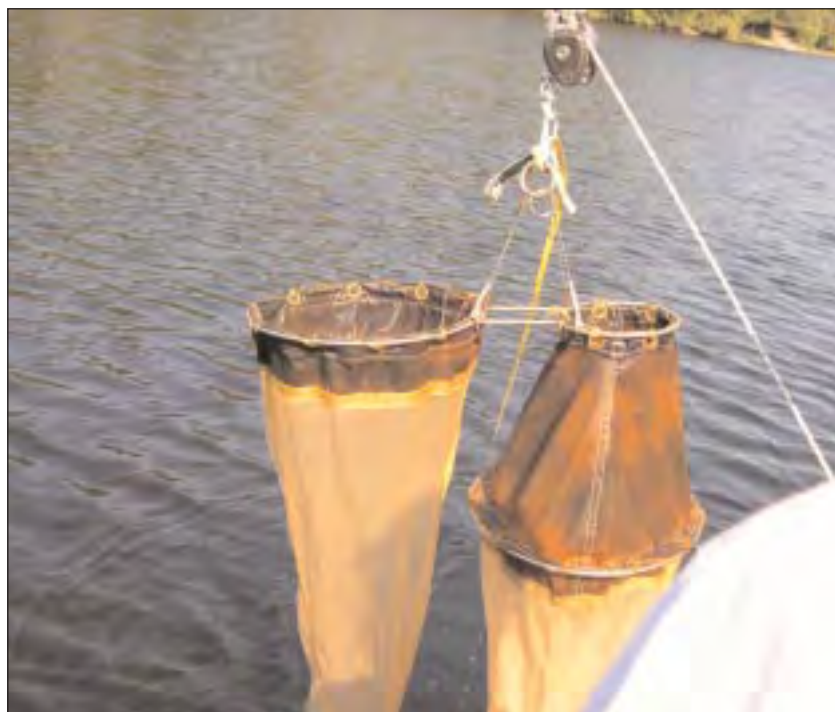
Netting the Evidence In the NELAP study, nets towed alongside a boat are used to collect plankton samples. Plankton are good indicators of ecosystem health because they are highly sensitive to environmental change, particularly nutrient enrichment.
