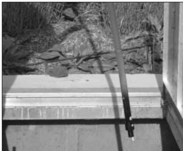
A sludge judge can be used to collect sludge samples.
