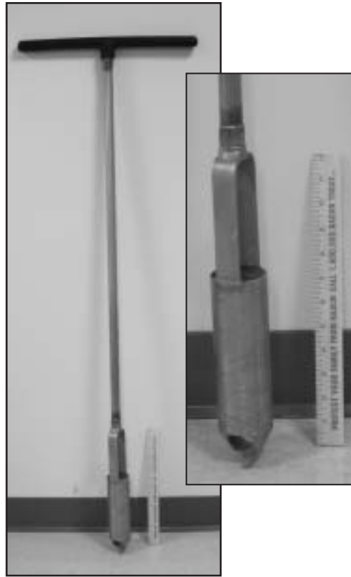
Soil Auger, note drill-like cutters
