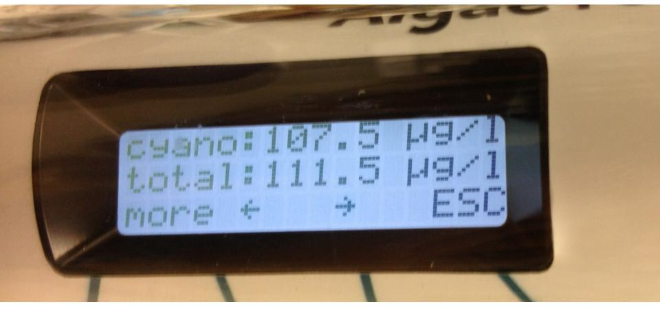
Best feature of the Algae Torch is that it gives rapid, relative percentages of cyanobacteria in the water. It can be used in the field along the shore or in the lab with a water sample.
